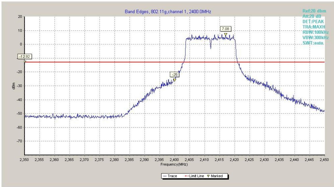
Fig.A.5.3 Band Edges (802.11g, Ch 1)
