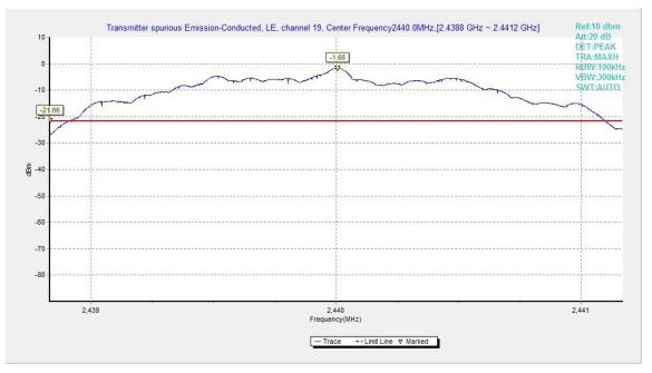
Fig.8. Transmitter Spurious Emission - Conducted: GFSK, 2440MHz
