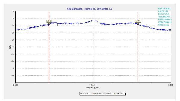
Fig.21. 6dB Bandwidth: GFSK, 2440 MHz
