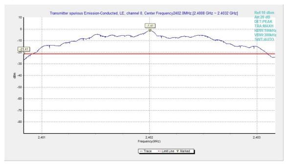
Fig.3. Transmitter Spurious Emission - Conducted: GFSK,2402MHz
