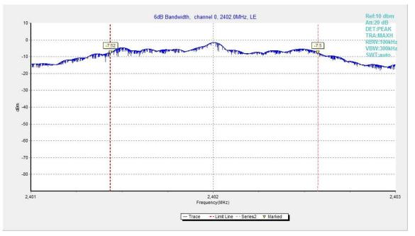
Fig.20. 6dB Bandwidth: GFSK, 2402 MHz
