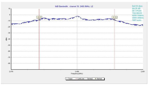
Fig.22. 6dB Bandwidth: GFSK, 2480 MHz
