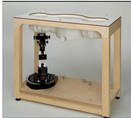
Picture C.10: SAM Twin Phantom
