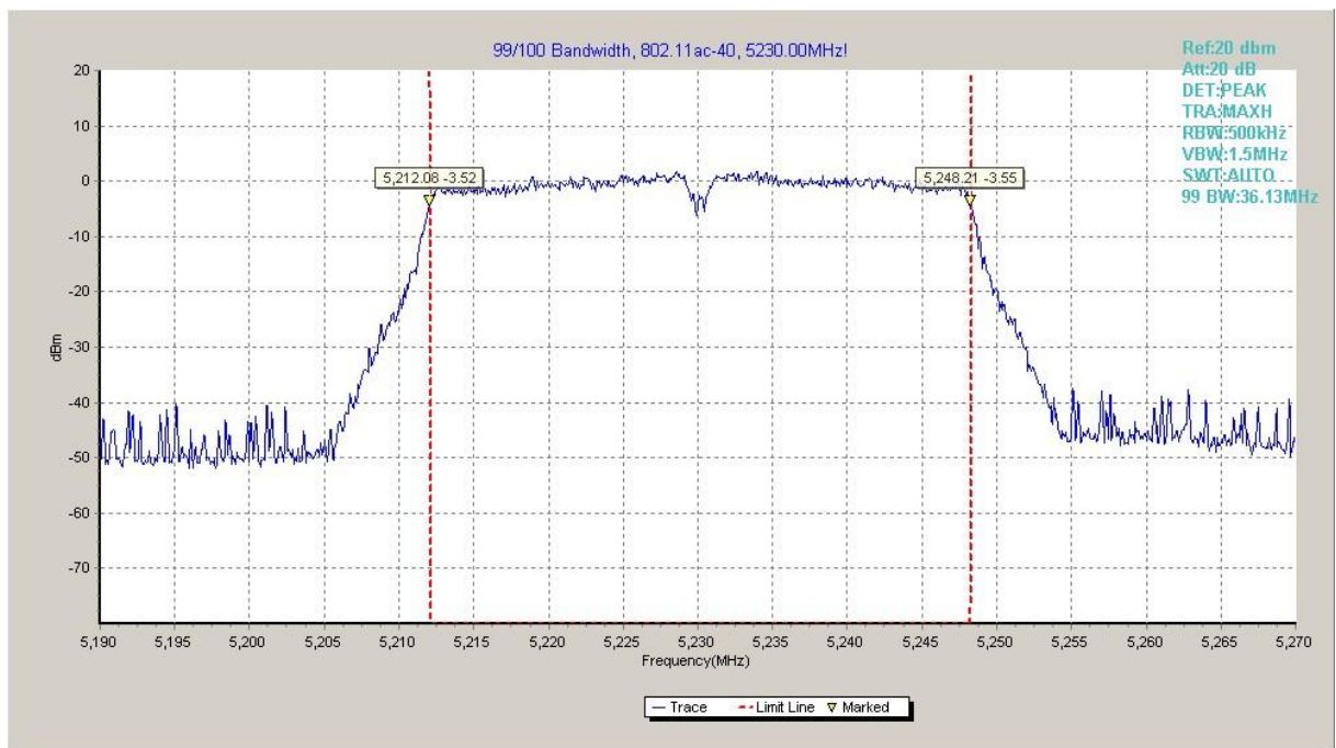
Fig. 83 99% Occupied bandwidth (802.11ac-HT40, 5230MHz)
