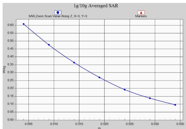
Fig.A.1- 3 Z-Scan at power reference point (PCS1900)
