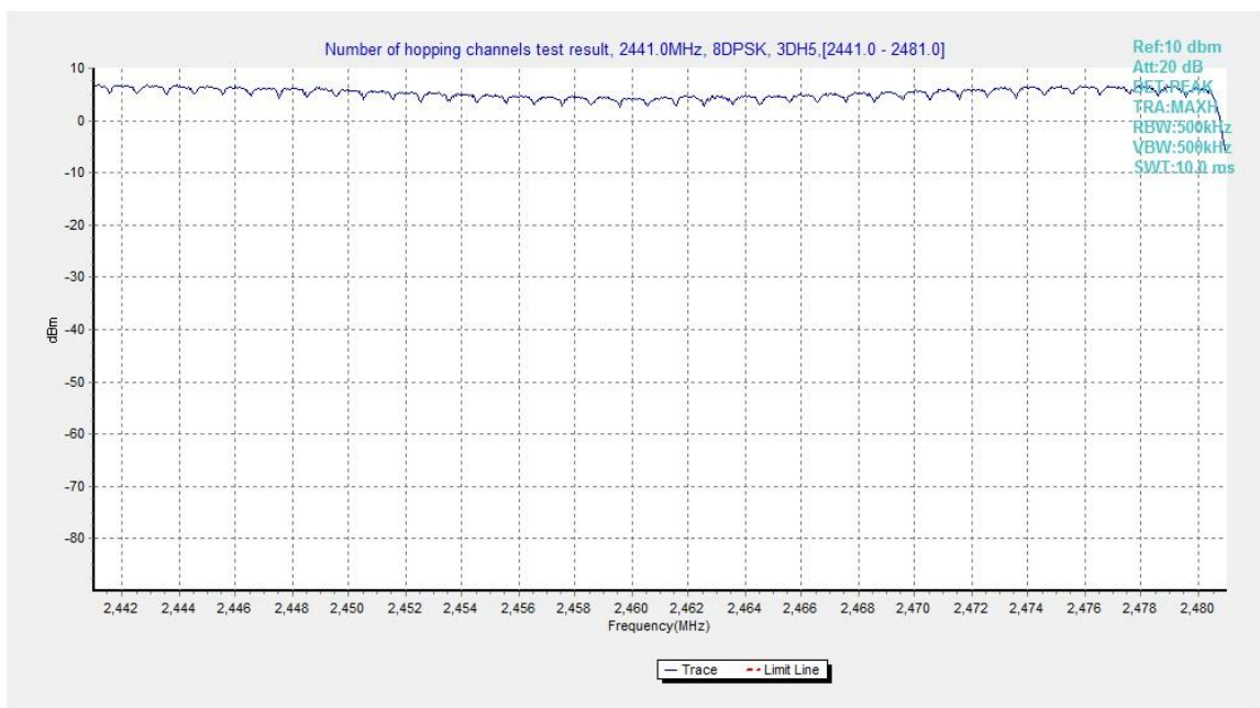
Fig.99. Number of hopping frequencies: 8DPSK, Channel 40 - 78
