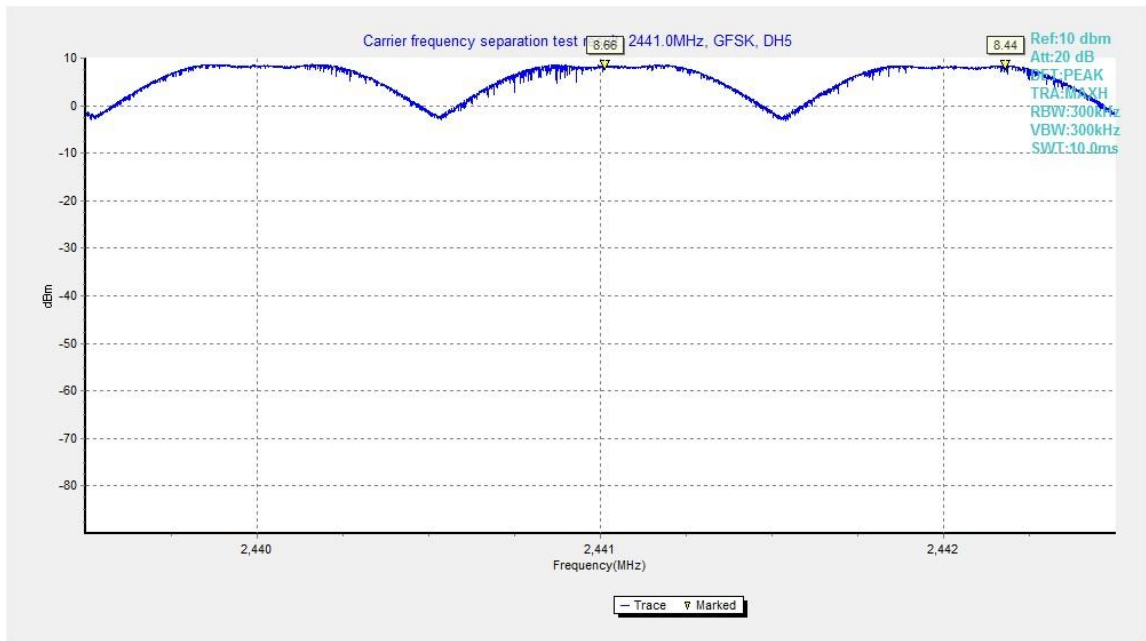
Fig.91. Carrier frequency separation measurement: GFSK, Channel 39
