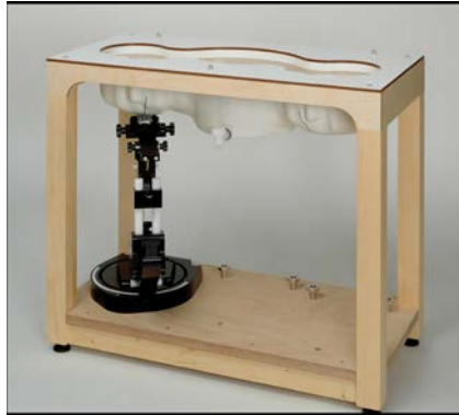
Picture C.10: SAM Twin Phantom
