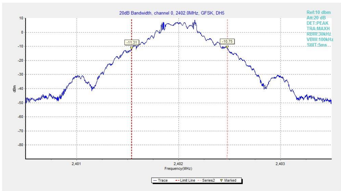
Fig.98. 20dB Bandwidth: GFSK, Channel 0
