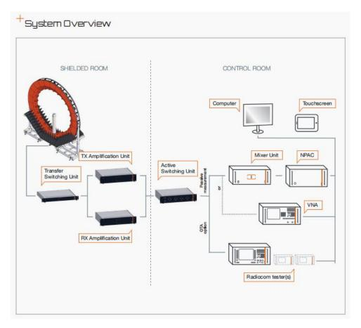
The figure above shows the connection and control process between the anechoic chamber of our company and the testing system and computer. The testing system has the characteristics of accurate, fast and simple testing. The operation interface is simple and humanized.
