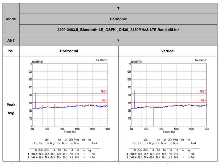
Note: For all plots above, the over limit line signals are Fundamental signal which can be ignored.
