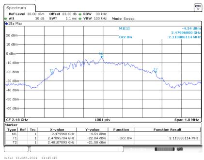
Note: The occupied channel bandwidth is maintained within the band of operation for all of the modulations.
