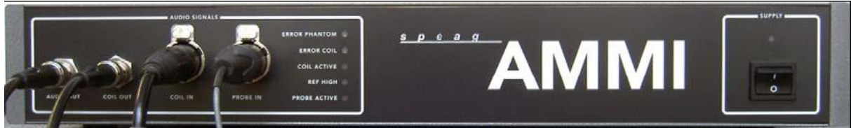
Figure 5.3 AMMI front panel
