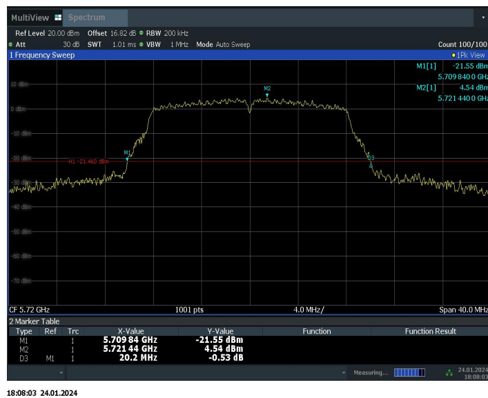
Fig.10 26dB Emission Bandwidth (802.11a, 5720MHz)
