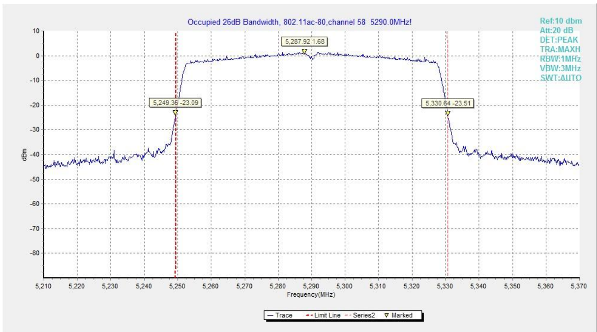
Fig.30 26dB Emission Bandwidth (802. 11ac-VHT80, 5290MHz)
