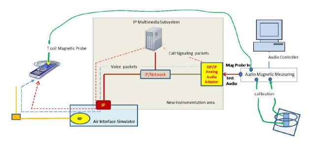
Figure 11.1 Test Setup for VoWiFi over IMS T-coil Measurements
