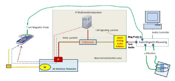
Figure 10.1 Test Setup for VoNR over IMS T-coil Measurements
