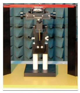
Figure 5.4 HAC Phantom & Device Holder
