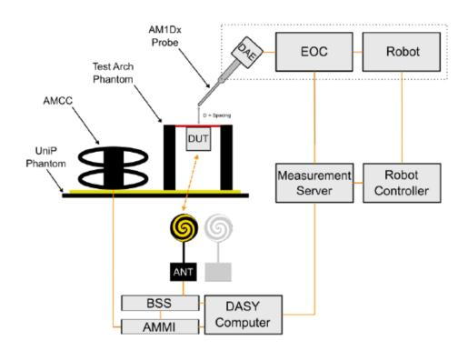
Figure 5.1 HAC Test Measurement Set-up
