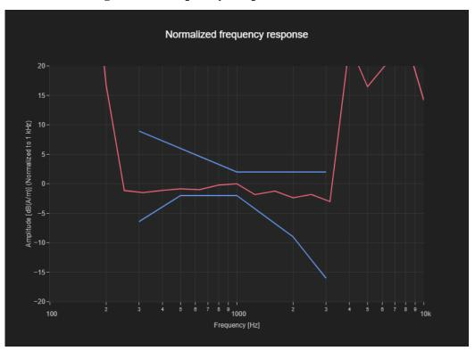
Figure C.4 Frequency Response of N25-0TT
