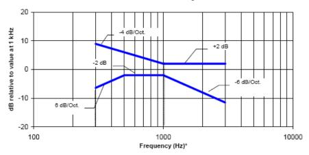
NOTE—Frequency response is between 300 Hz and 3000 Hz.
