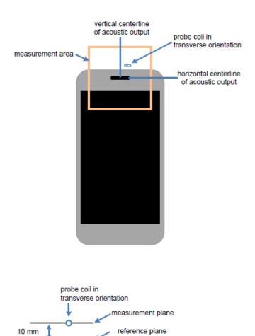
Figure 5.5 Measurement and reference planes probe orientation for WD audio frequency magnetic field measurements
