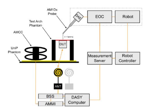
Figure 5.1 HAC Test Measurement Set-up
