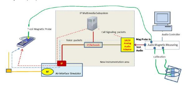
Figure 9.1 Test Setup for VoLTE over IMS T-coil Measurements
