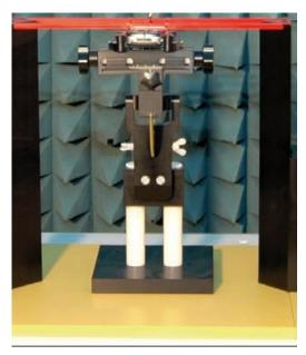
Figure 5.4 HAC Phantom & Device Holder
