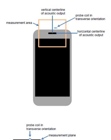
Figure 5.5 Measurement and reference planes probe orientation for WD audio frequency magnetic field measurements
