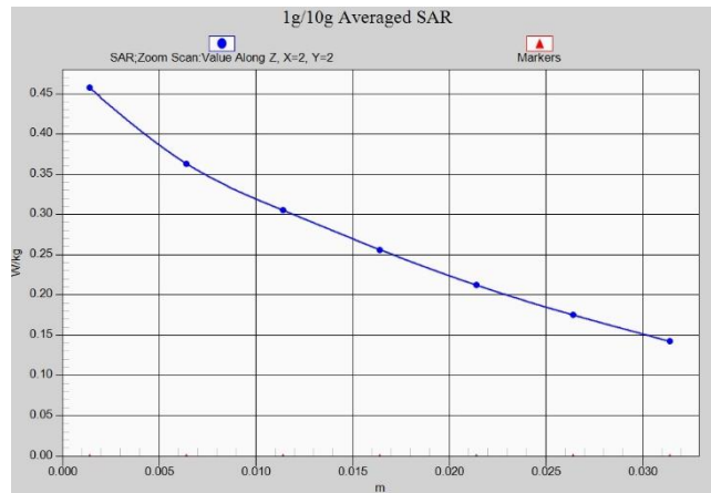
Z-Scan at power reference point (LTEB13)
