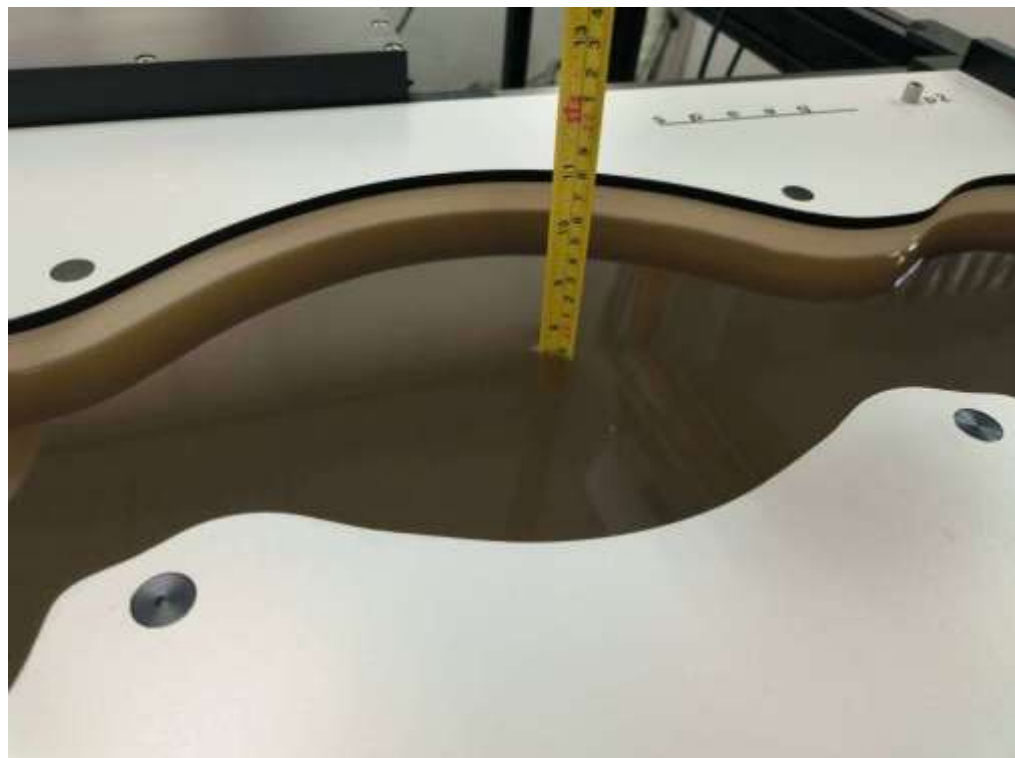
Picture 7-2 Liquid depth in the Body Phantom
