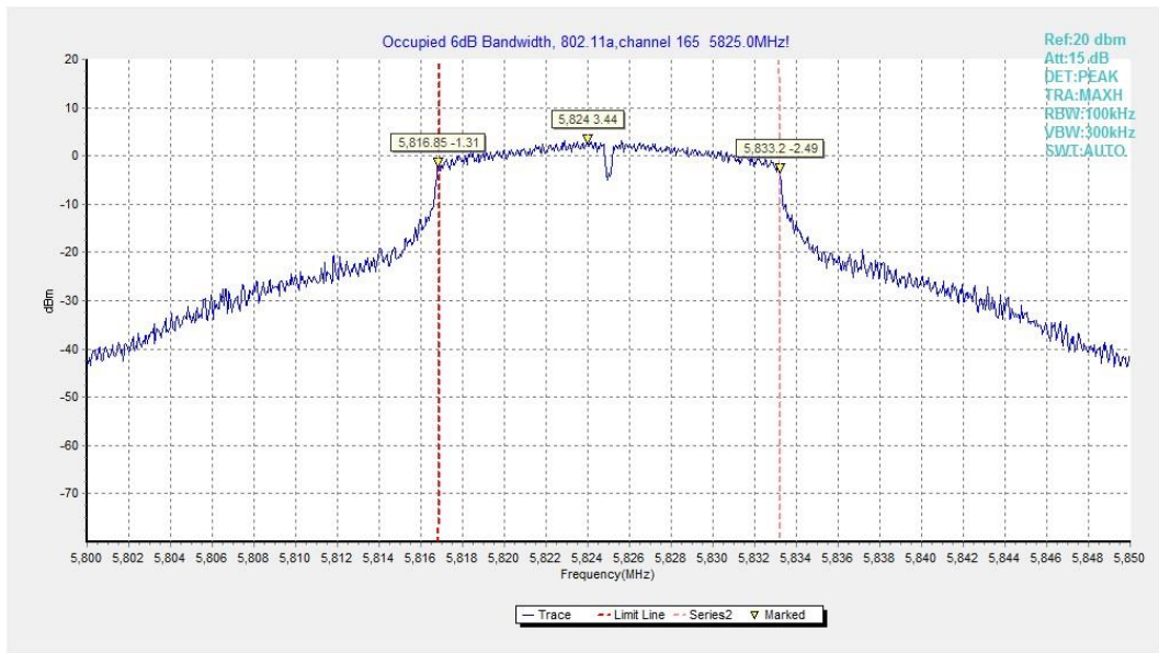
Fig. 3 Occupied 6dB Bandwidth (802.11a, Ch 165)
