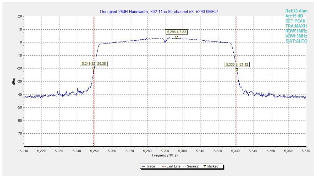
Fig.30 Occupied 26dB Bandwidth (802.11ac-HT80, 5290MHz)
