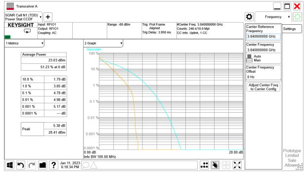
n77H, 100MHz Bandwidth, DFT-s-QPSK (PAPR)
