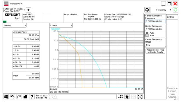
n78H, 100MHz Bandwidth, DFT-s-QPSK (PAPR)
