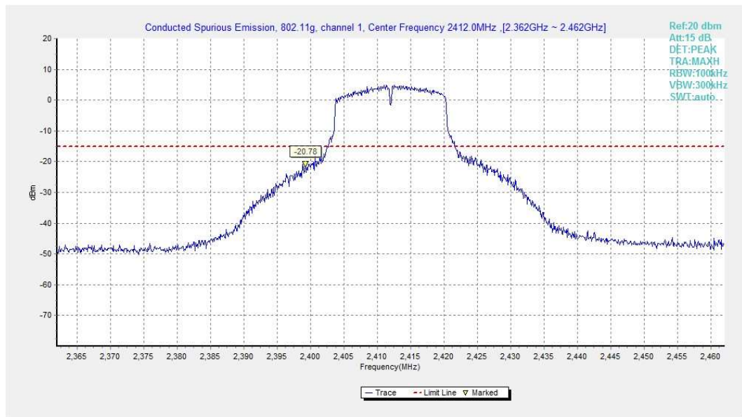
Fig.A.6.1.25 Transmitter Spurious Emission - Conducted (802.11g, Ch1, Center Frequency)
