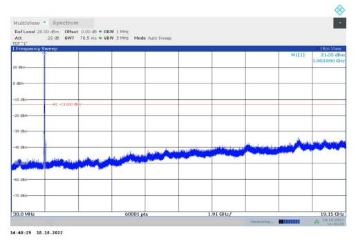
n41 NOTE: peak above the limit line is the carrier frequency.
