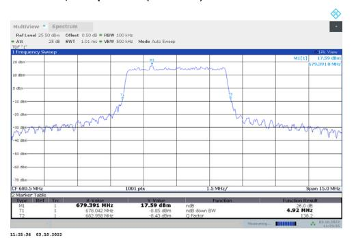
n71,5MHz Bandwidth,DFT-s-QPSK (-26dBc BW)
