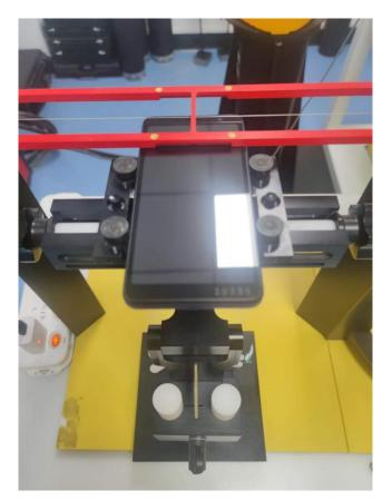
Picture 2: EUT Positioning for RF/T-coil
