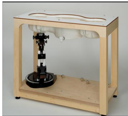
Picture C.8: SAM Twin Phantom
