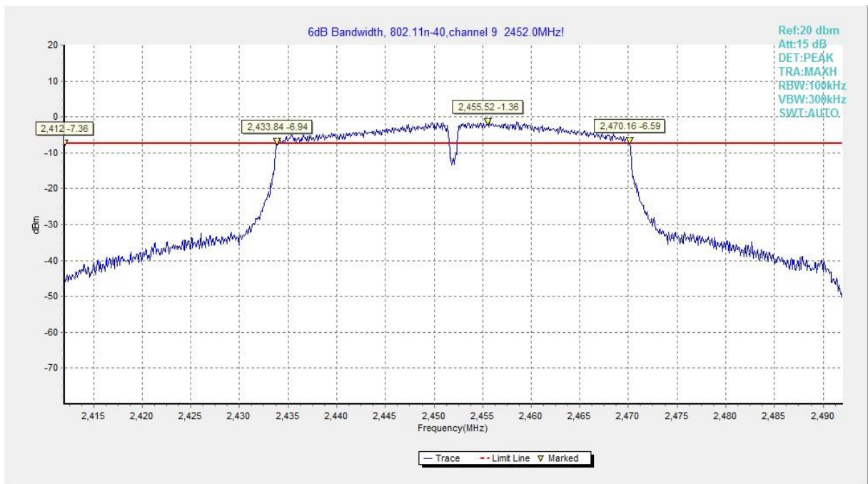
Fig.A.4.12 Occupied 6dB Bandwidth (802.11n-HT40, Ch 9)
