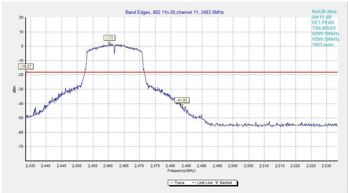
Fig.A.5.6 Band Edges (802.11n-HT20, Ch 11)
