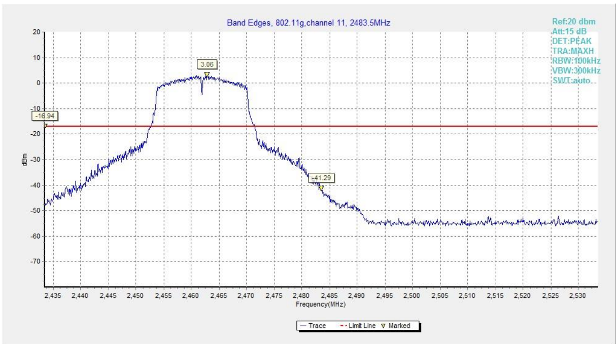
Fig.A.5.4 Band Edges (802.11g, Ch 11)
