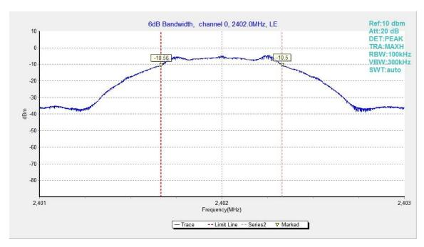
Fig.20. 6dB Bandwidth: GFSK, 2402 MHz
