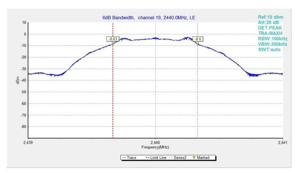
Fig.21. 6dB Bandwidth: GFSK, 2440 MHz
