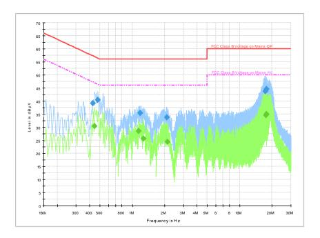
Fig.B.9.2 AC Powerline Conducted Emission-Idle
