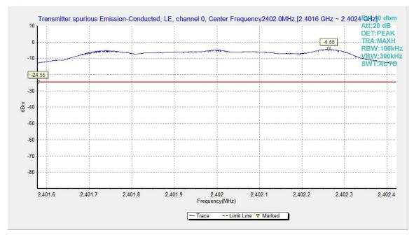
Fig.5. Transmitter Spurious Emission - Conducted: GFSK,2402MHz
