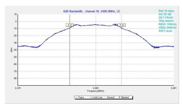
Fig.22. 6dB Bandwidth: GFSK, 2480 MHz
