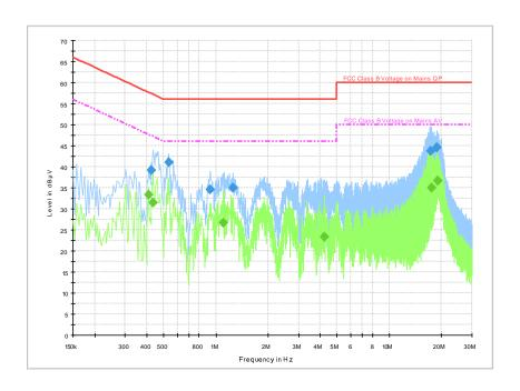
Fig.B.9.1 AC Powerline Conducted Emission- bluetooth
