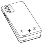
Insert the battery by connecting the gold contacts in the device battery cavity. The battery will only fit one way.
