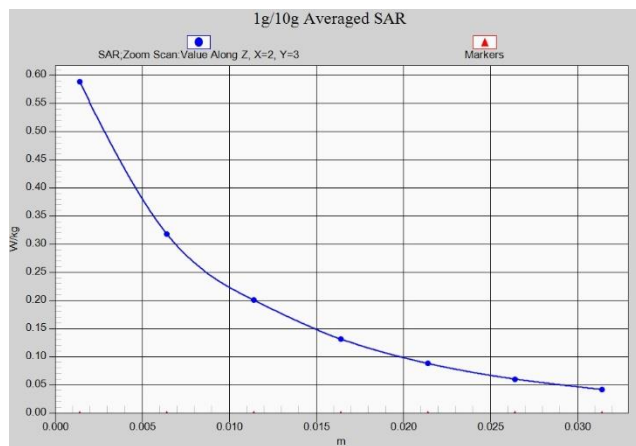
Z-Scan at power reference point (LTEB13)
