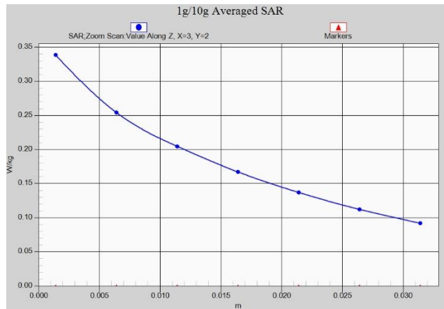
Z-Scan at power reference point (LTEB13)
