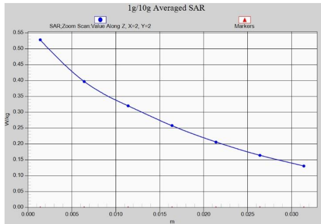
Z-Scan at power reference point (LTEB26)
