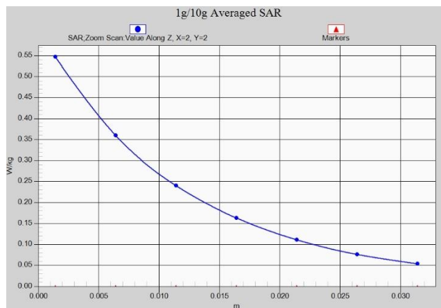
Z-Scan at power reference point (LTEB66)
