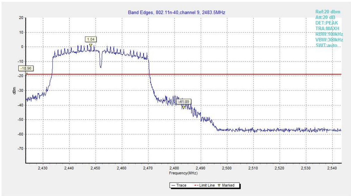
Fig.32 Band Edges (802.11n HT40, CH 9)
