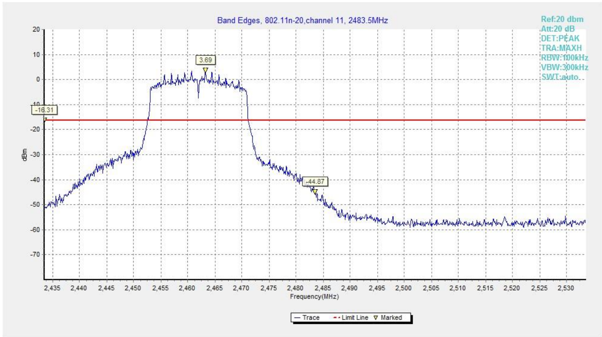
Fig.30 Band Edges (802.11n HT20, CH 11)
