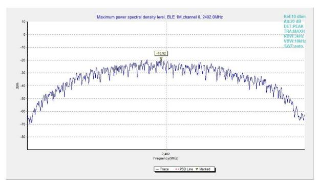
Fig.1 Power Spectral Density (Ch 0), LE 1M
