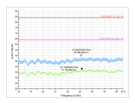
Fig.51 Radiated Spurious Emission (Ch19, 18 GHz - 26.5 GHz), 2M
