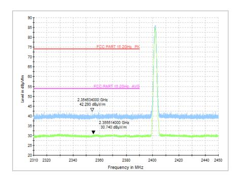
Fig.45 Radiated Band Edges (Ch0, 2380GHz - 2450GHz), 1M
