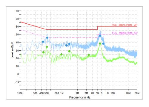
Fig.56 AC Power line Conducted Emission (Idle, AE2, 120V), 1M
