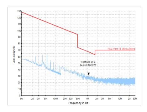
Fig.40 Radiated Spurious Emission (Ch19, 9 kHz - 30 MHz), 1M
