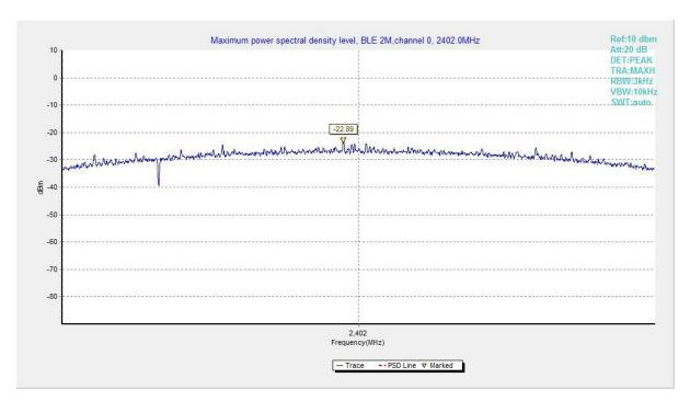
Fig.4 Power Spectral Density (Ch 0), LE 2M
