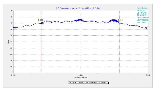
Fig.11 6dB Bandwidth (Ch 19), LE 2M
