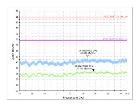
Fig.43 Radiated Spurious Emission (Ch19, 18 GHz - 26.5 GHz), 1M
