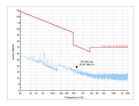
Fig.48 Radiated Spurious Emission (Ch19, 9 kHz - 30 MHz), 2M
