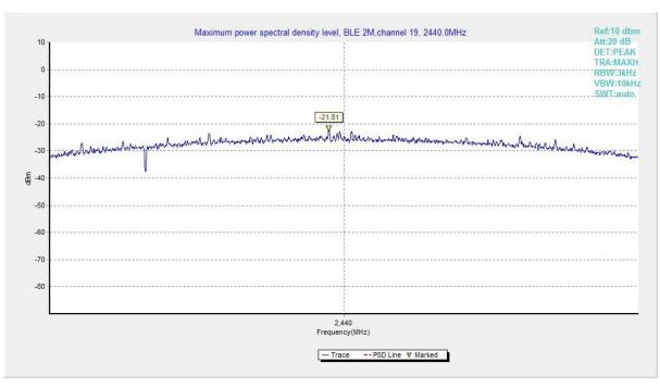
Fig.5 Power Spectral Density (Ch 19), LE 2M
