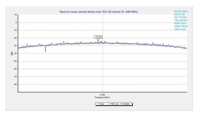
Fig.6 Power Spectral Density (Ch 39), LE 2M
