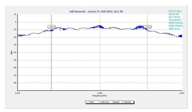
Fig.12 6dB Bandwidth (Ch 39), LE 2M
