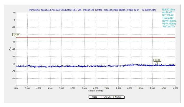
Fig.36 Conducted Spurious Emission (Ch39, 3 GHz-10 GHz), LE 2M
