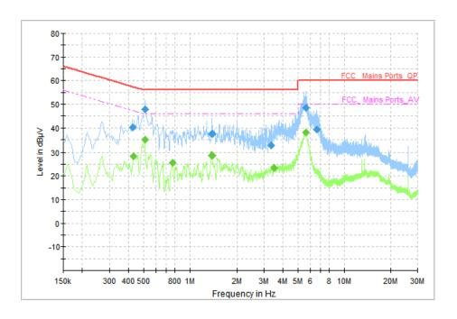
Fig.57 AC Power line Conducted Emission (Traffic, AE2, 120V), 2M
