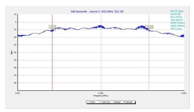
Fig.10 6dB Bandwidth (Ch 0), LE 2M
