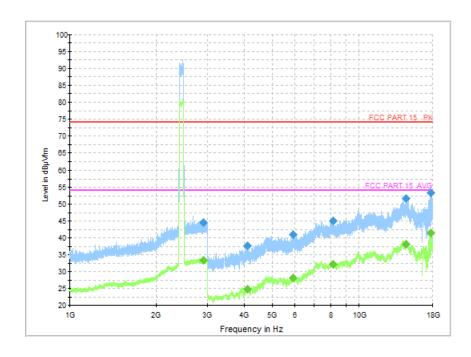
Fig.42 Radiated Spurious Emission (Ch19, 1 GHz - 18 GHz), 1M
