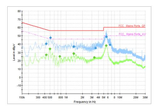
Fig.58 AC Power line Conducted Emission (Idle, AE2, 120V), 2M
