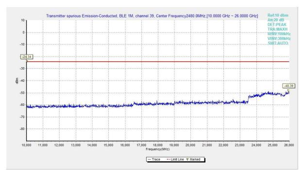
Fig.27 Conducted Spurious Emission (All channels, 10 GHz-26 GHz), LE 1M
