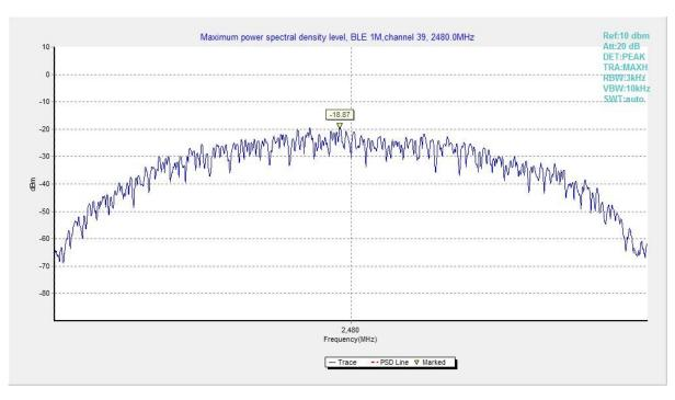
Fig.3 Power Spectral Density (Ch 39), LE 1M
