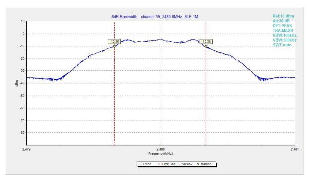
Fig.9 6dB Bandwidth (Ch 39), LE 1M
