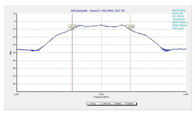
Fig.7 6dB Bandwidth (Ch 0), LE 1M
