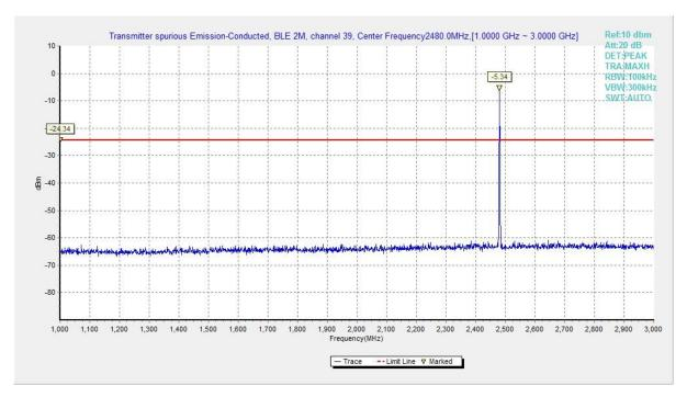
Fig.35 Conducted Spurious Emission (Ch39, 1 GHz-3 GHz), LE 2M
