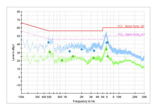
Fig.55 AC Power line Conducted Emission (Traffic, AE2, 120V), 1M
