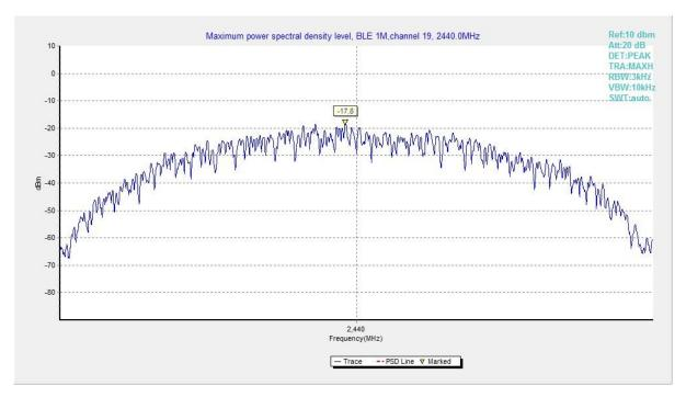
Fig.2 Power Spectral Density (Ch 19), LE 1M
