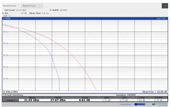
LTE band 26(824MHz -849MHz), 10MHz Bandwidth, 16QAM (PAPR)
