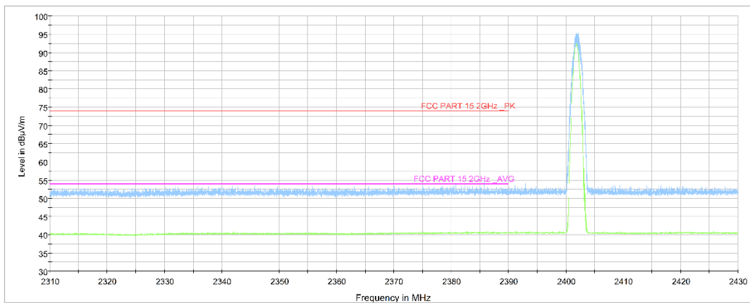
Fig.15. Frequency Band Edges: \pi/4 DQPSK, Channel 0, Hopping Off, 2.31GHz ~2.43GHz
