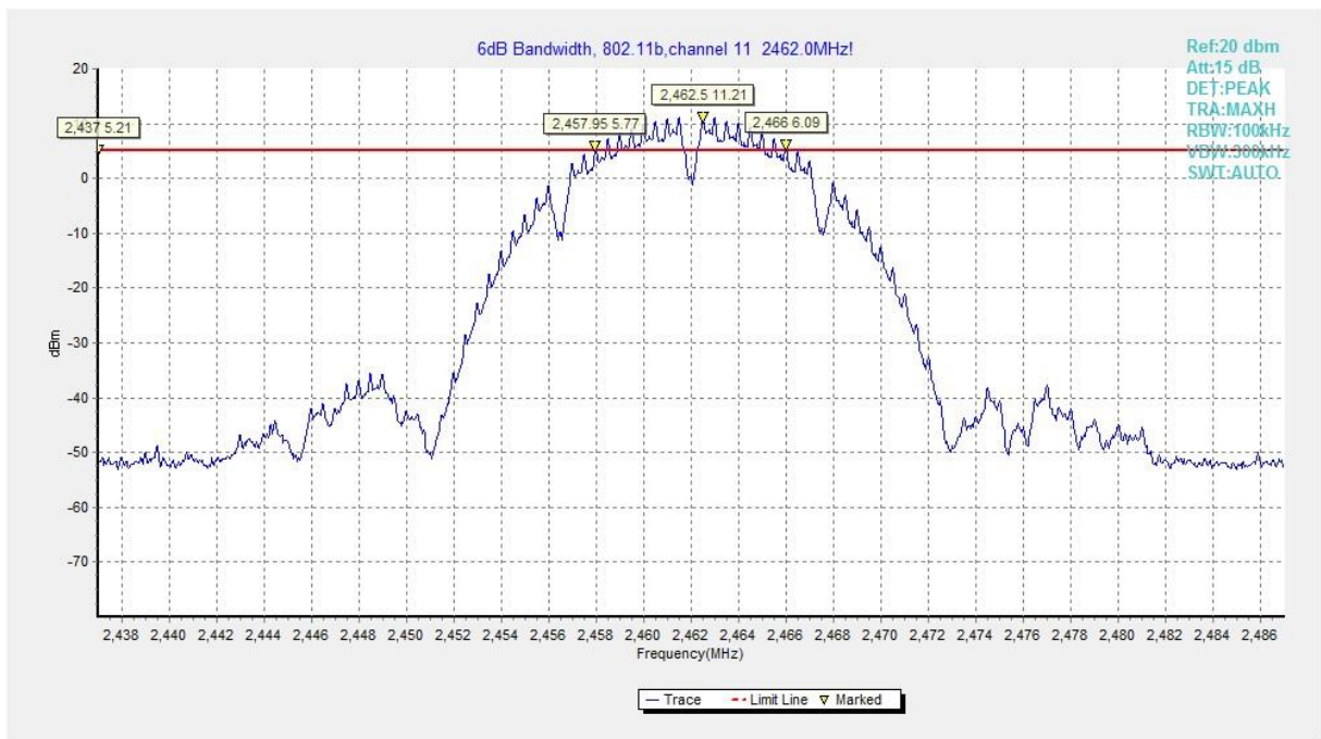
Fig.A.4.3 Occupied 6dB Bandwidth (802.11b, Ch 11)
