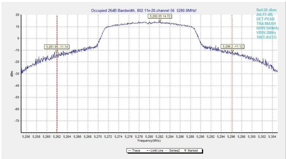
Fig.15 Occupied 26dB Bandwidth (802.11n-HT20, 5280MHz)
