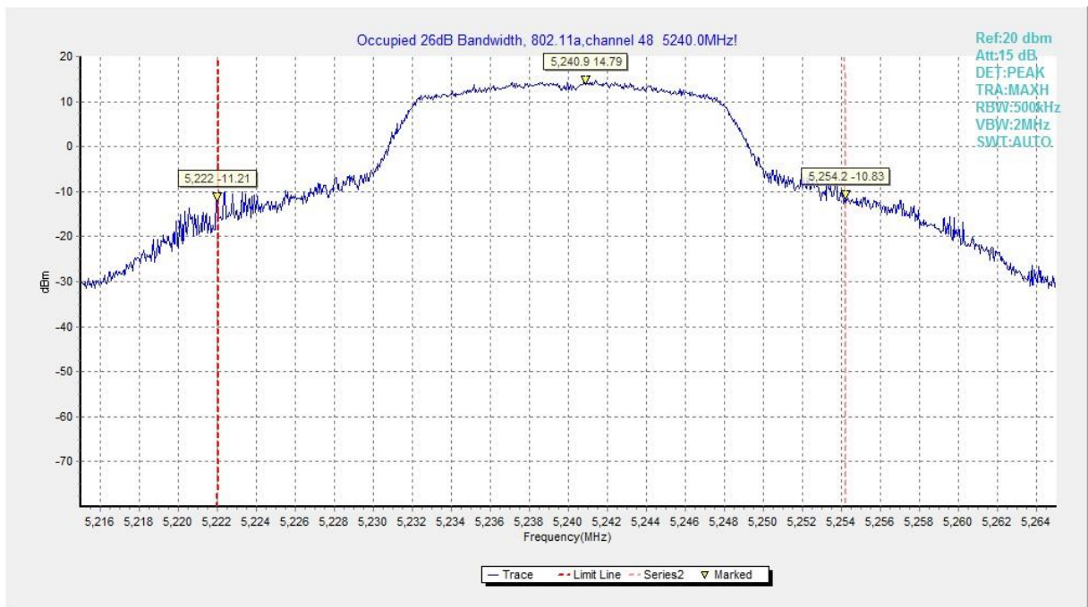
Fig.3 Occupied 26dB Bandwidth (802.11a, 5240MHz)
