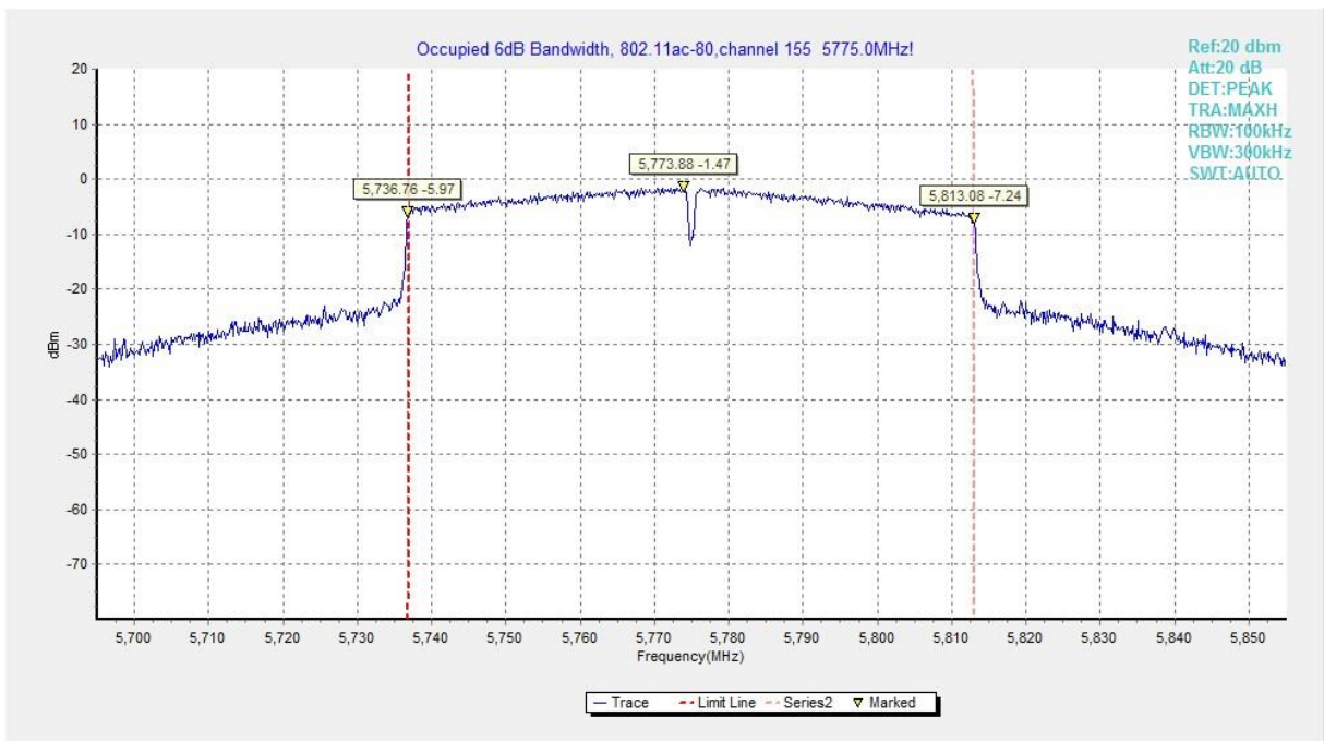
Fig. 9 Occupied 6dB Bandwidth (802.11ac-HT80, Ch 155)
