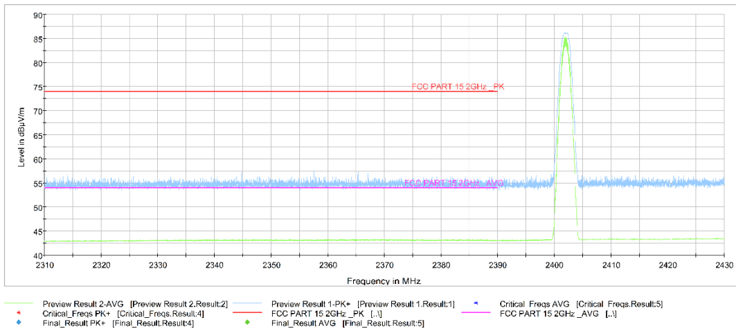
Fig.3. Frequency Band Edges: GFSK, 2402 MHz, Hopping Off, 2.31 GHz – 2.43GHz
