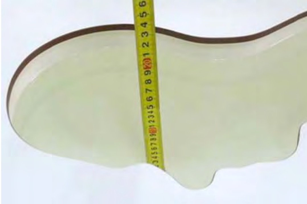
Picture 3: liquid depth in the head Phantom
