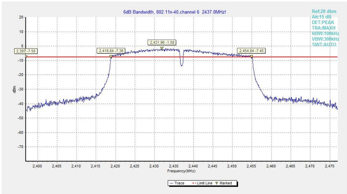
Fig.A.4.11 Occupied 6dB Bandwidth (802.11n-HT40, Ch 6)
