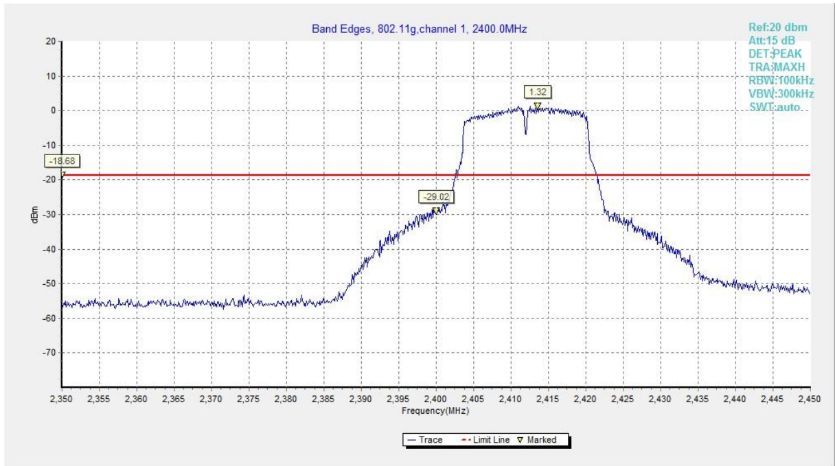
Fig.A.5.3 Band Edges (802.11g, Ch 1)
