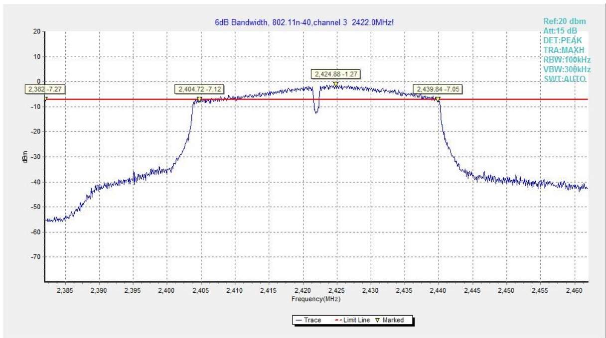
Fig.A.4.10 Occupied 6dB Bandwidth (802.11n-40MHz, Ch 3)
