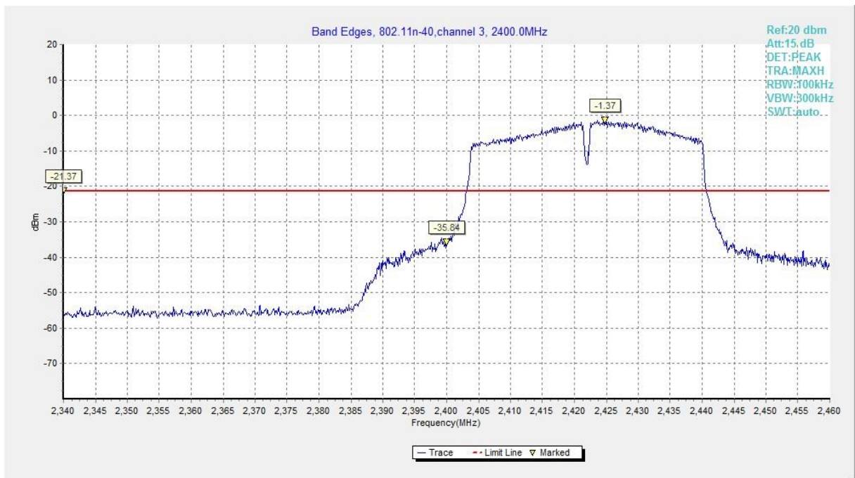
Fig.A.5.7 Band Edges (802.11n-HT40, Ch 3)
