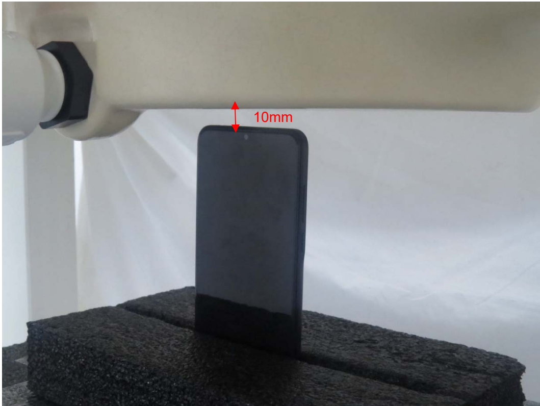
Picture 11: Top Edge, the distance from handset to the bottom of the Phantom is 10mm
