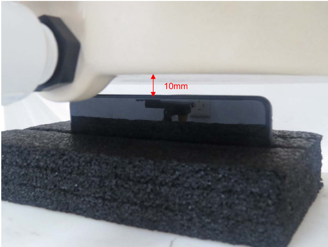
Picture 9: Left Edge, the distance from handset to the bottom of the Phantom is 10mm
