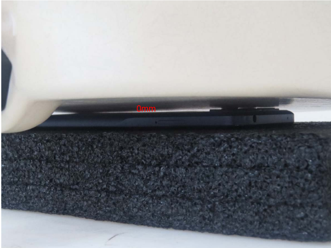
Picture 13: Back Side, the distance from handset to the bottom of the Phantom is 0mm
