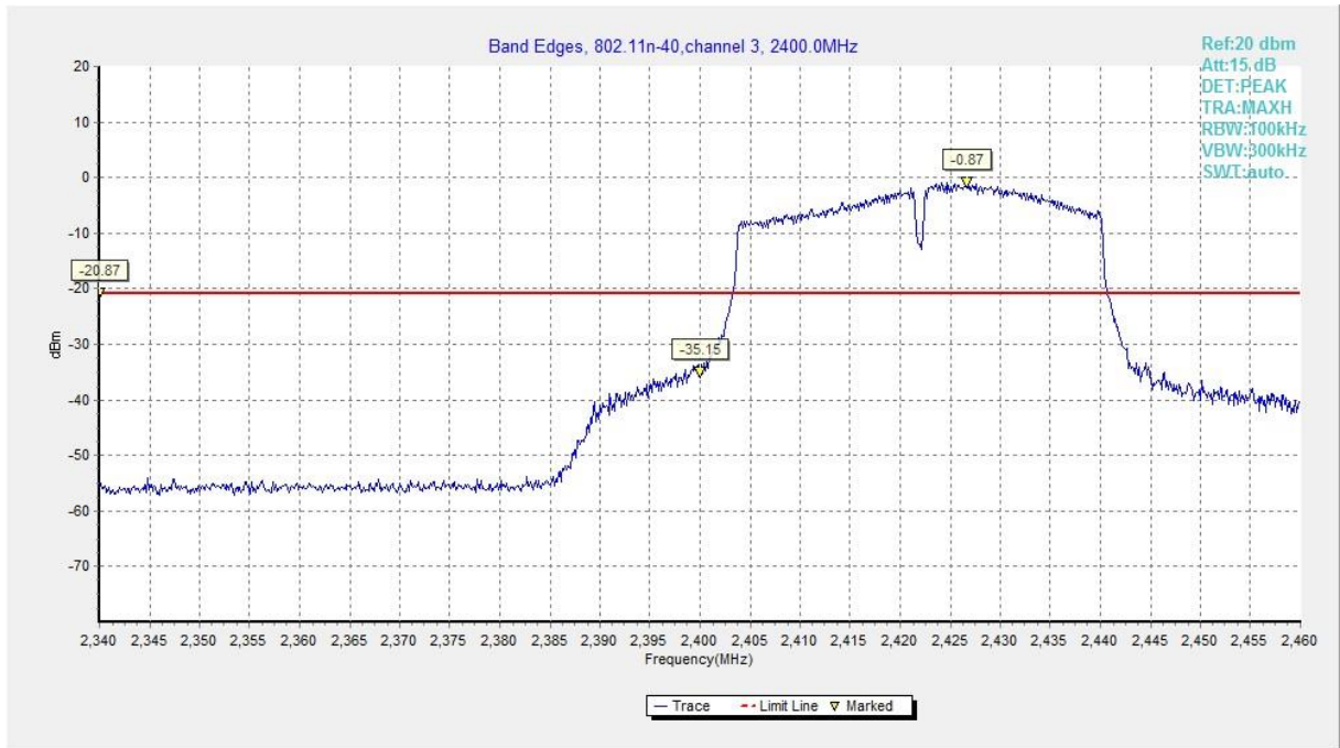
Fig.A.5.7 Band Edges (802.11n-HT40, Ch 3)
