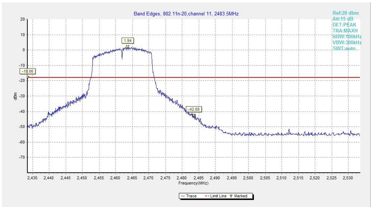
Fig.A.5.6 Band Edges (802.11n-HT20, Ch 11)
