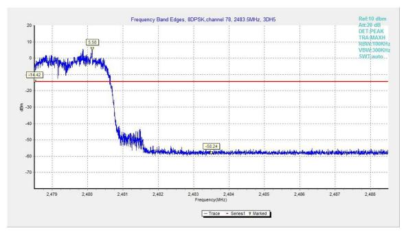
Fig.12. Frequency Band Edges: 8DPSK, Channel 78, Hopping On
