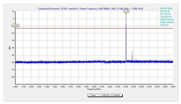
Fig.21. Conducted spurious emission: GFSK, Channel 0, 1GHz - 3GHz
