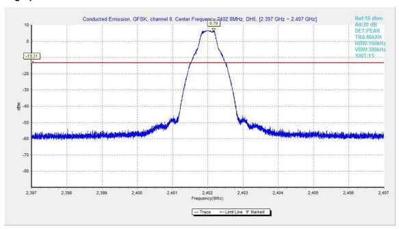
Fig.19. Conducted spurious emission: GFSK, Channel 0,2402MHz
