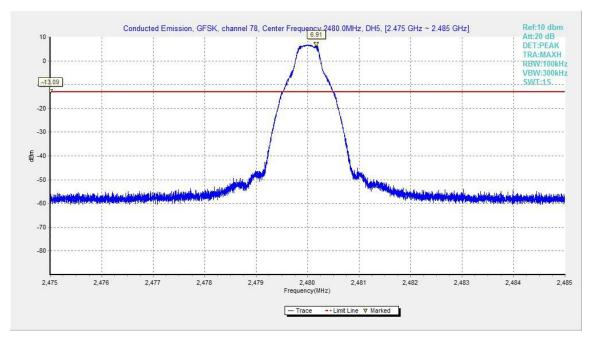
Fig.29. Conducted spurious emission: GFSK, Channel 78, 2480MHz
