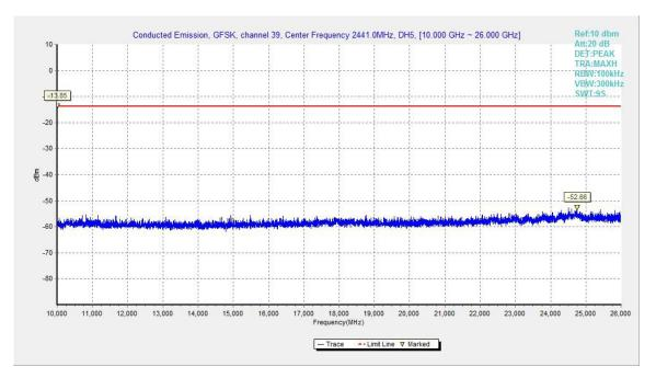
Fig.28. Conducted spurious emission: GFSK, Channel 39, 10GHz – 26GHz
