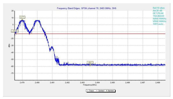
Fig.4. Frequency Band Edges: GFSK, Channel 78, Hopping On
