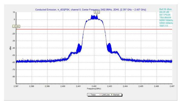
Fig.34. Conducted spurious emission: π/4 DQPSK, Channel 0,2402MHz
