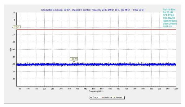
Fig.20. Conducted spurious emission: GFSK, Channel 0, 30MHz - 1GHz
