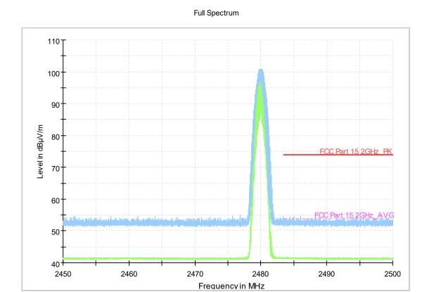
Fig.16. Frequency Band Edges: π/4 DQPSK, Channel 78, Hopping Off, 2.38 GHz - 2.45GHz
