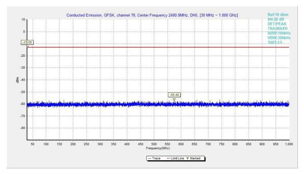
Fig.30. Conducted spurious emission: GFSK, Channel 78, 30MHz - 1GHz
