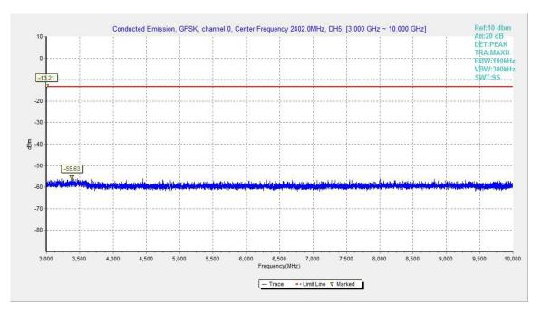
Fig.22. Conducted spurious emission: GFSK, Channel 0, 3GHz - 10GHz
