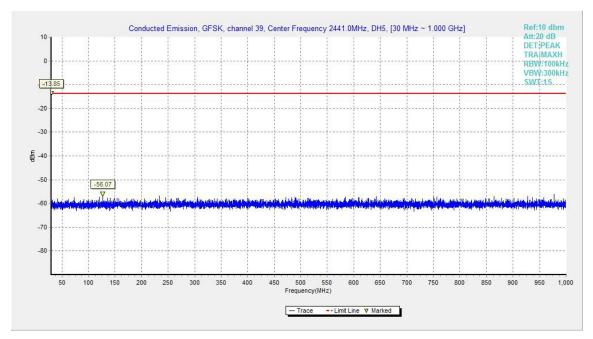
Fig.25. Conducted spurious emission: GFSK, Channel 39, 30MHz - 1GHz
