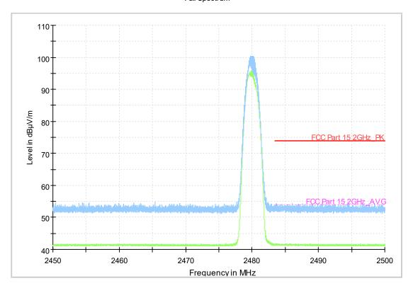
Fig.18. Frequency Band Edges: 8DPSK, Channel 78, 2.38 GHz - 2.45GHz
