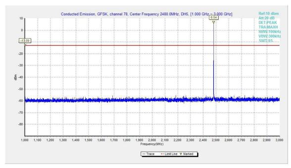
Fig.31. Conducted spurious emission: GFSK, Channel 78, 1GHz - 3GHz
