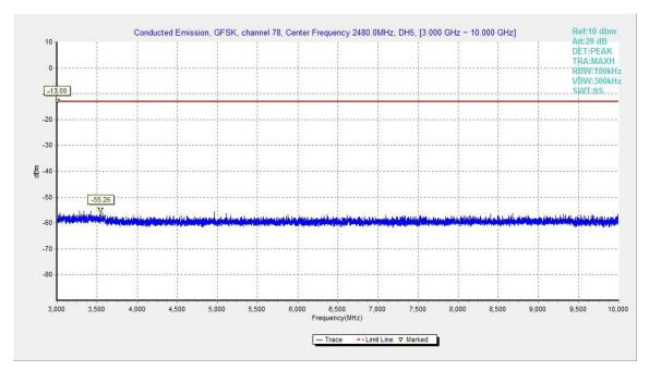
Fig.32. Conducted spurious emission: GFSK, Channel 78, 3GHz - 10GHz
