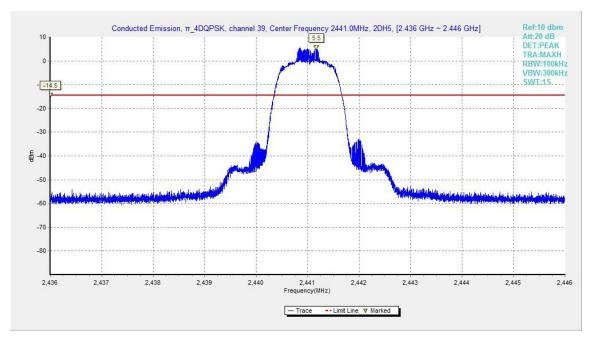
Fig.39. Conducted spurious emission:  $\pi/4$  DQPSK, Channel 39, 2441MHz
