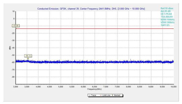
Fig.27. Conducted spurious emission: GFSK, Channel 39, 3GHz – 10GHz
