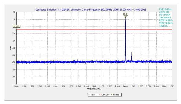
Fig.36. Conducted spurious emission: π/4 DQPSK, Channel 0, 1GHz - 3GHz
