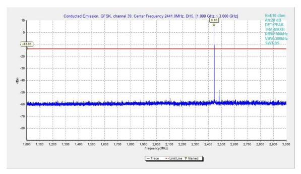
Fig.26. Conducted spurious emission: GFSK, Channel 39, 1GHz – 3GHz
