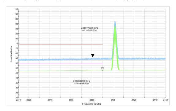
Fig.17. Frequency Band Edges: 8DPSK, Channel 0, 2.38 GHz - 2.45GHz
