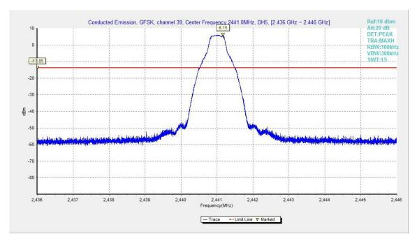
Fig.24. Conducted spurious emission: GFSK, Channel 39, 2441MHz
