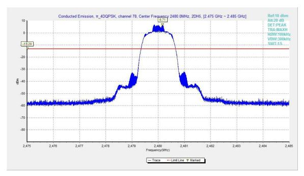
Fig.44. Conducted spurious emission:  $\pi/4$  DQPSK, Channel 78, 2480MHz
