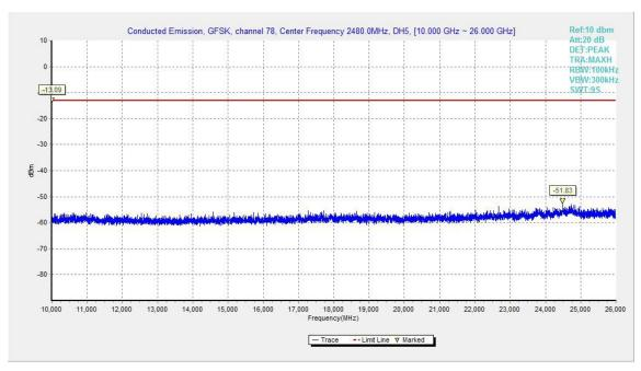
Fig.33. Conducted spurious emission: GFSK, Channel 78, 10GHz - 26GHz
