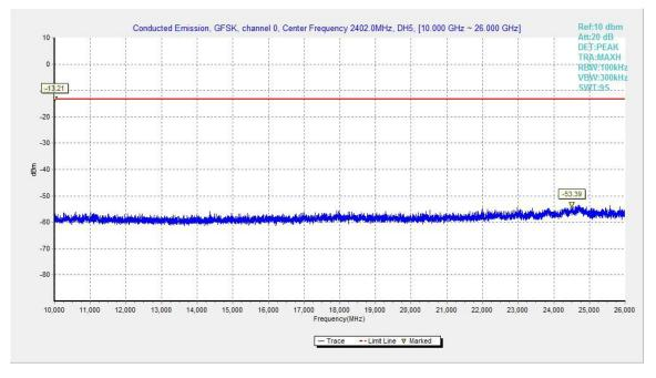
Fig.23. Conducted spurious emission: GFSK, Channel 0,10GHz - 26GHz
