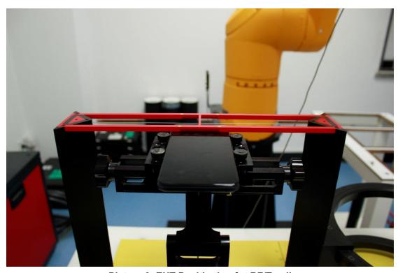
Picture 2: EUT Positioning for RF/T-coil
