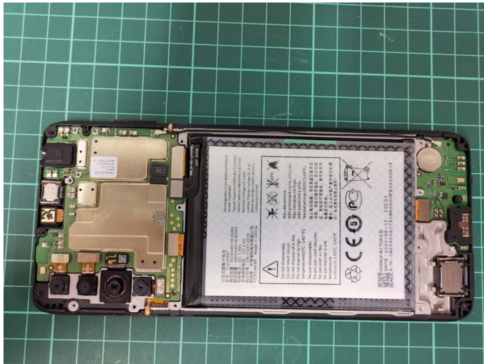
Mobile Phone Disassembly
