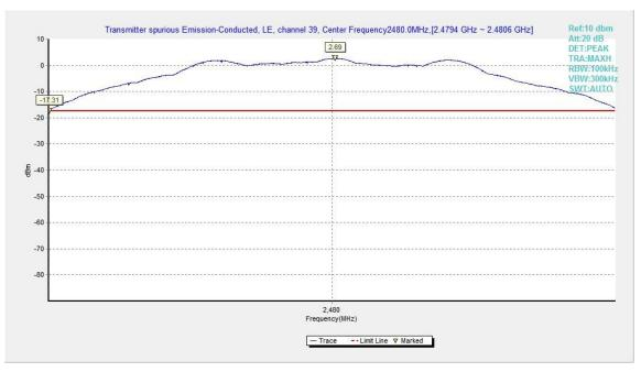
Fig.15. Transmitter Spurious Emission - Conducted: GFSK, 2480 MHz
