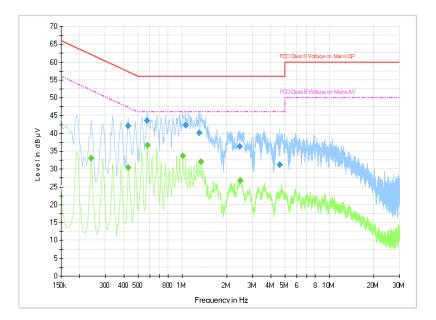
**Fig.B.9.4** AC Powerline Conducted Emission with Charger AE6-Idle Note: The graphic result above is the maximum of the measurements for both phase line and neutral line.
