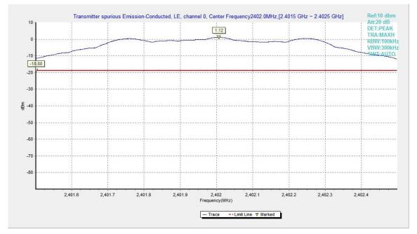
Fig.5. Transmitter Spurious Emission - Conducted: GFSK,2402MHz
