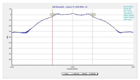
Fig.21. 6dB Bandwidth: GFSK, 2440 MHz
