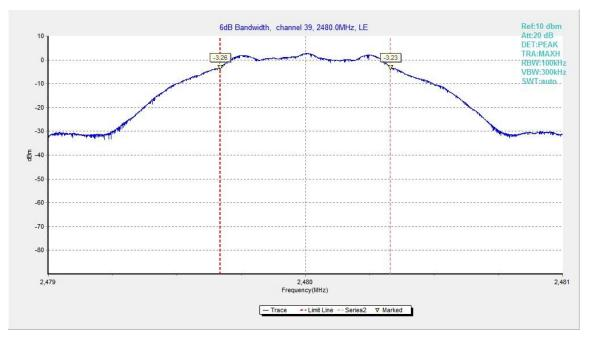
Fig.22. 6dB Bandwidth: GFSK, 2480 MHz
