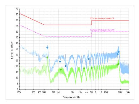
Fig.B.9.7AC Powerline Conducted Emission with Charger AE8- bluetoothNote: The graphic result above is the maximum of the measurements for both phase line and<br/>neutral line.
