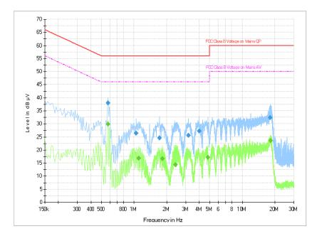
**Fig.B.9.8** AC Powerline Conducted Emission with Charger AE8-Idle Note: The graphic result above is the maximum of the measurements for both phase line and neutral line.
