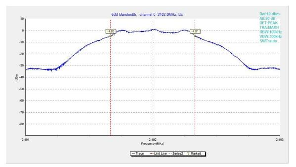
Fig.20. 6dB Bandwidth: GFSK, 2402 MHz
