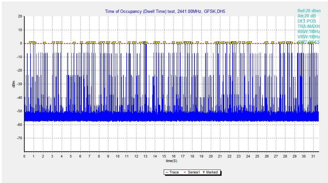
Fig.69. Number of Transmissions Measurement: Channel 39,Packet DH5
