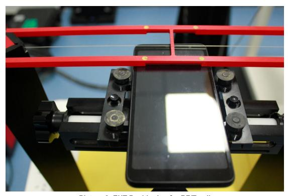
Picture 2: EUT Positioning for RF/T-coil
