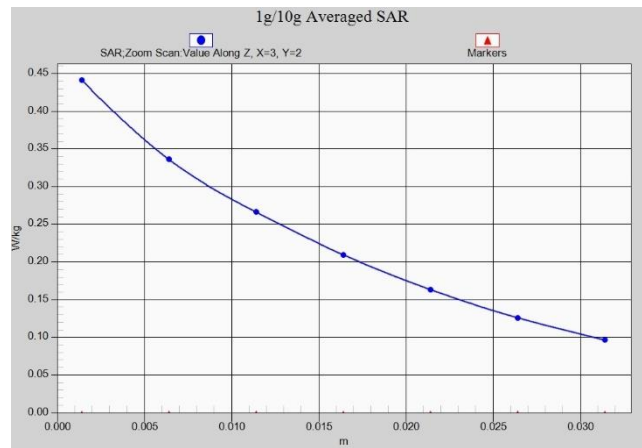
Fig. 1-22 Z-Scan at power reference point (LTEB26)
