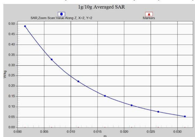
Fig. 1-29 Z-Scan at power reference point (LTEB66)
